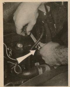
• SO THAT excessive wear will not develop in the camshaft, take care not to overtighten the cam chain. To make this adjustment, release the locking nut on the offside of the head, and turn the knurled screw with a spanner, as shown
