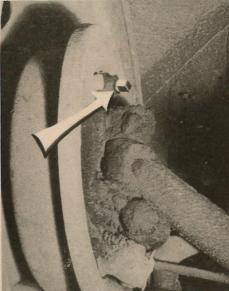
ADJUSTMENTS to the brakes to compensate for lining wear are executed by turning the square-headed nut at top of the drum backplate. It is quite unnecessary, even undesirable, to jack up the car to do this maintenance job.
